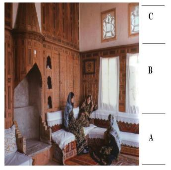
Figure 2. The room of a traditional Turkish house is shaped around divan- furnace- closet [3]. Interior space of room is vertically divided into three parts with respect to function, ergonomics and material application: A. Life surrounding, B. Accessible surrounding, C. Rarely used surrounding.
